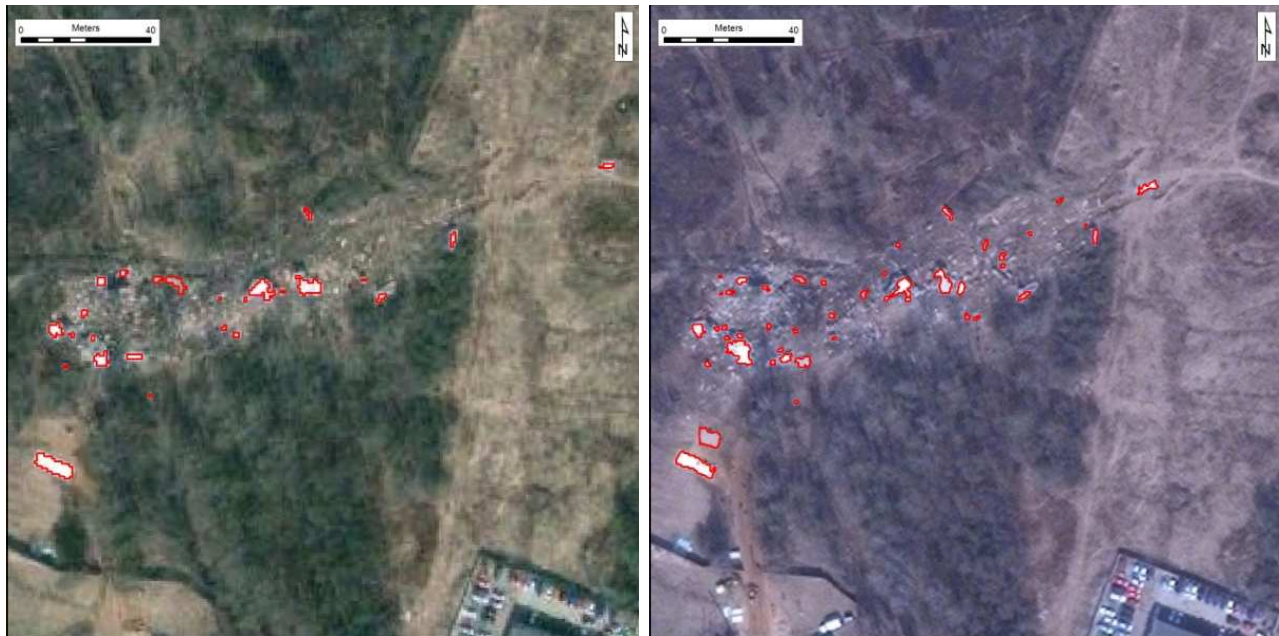
Figure 12: Trained auto-selection of polygons on the crash area sends up selecting most of the bigger parts scattered mainly around the perim of the site.
